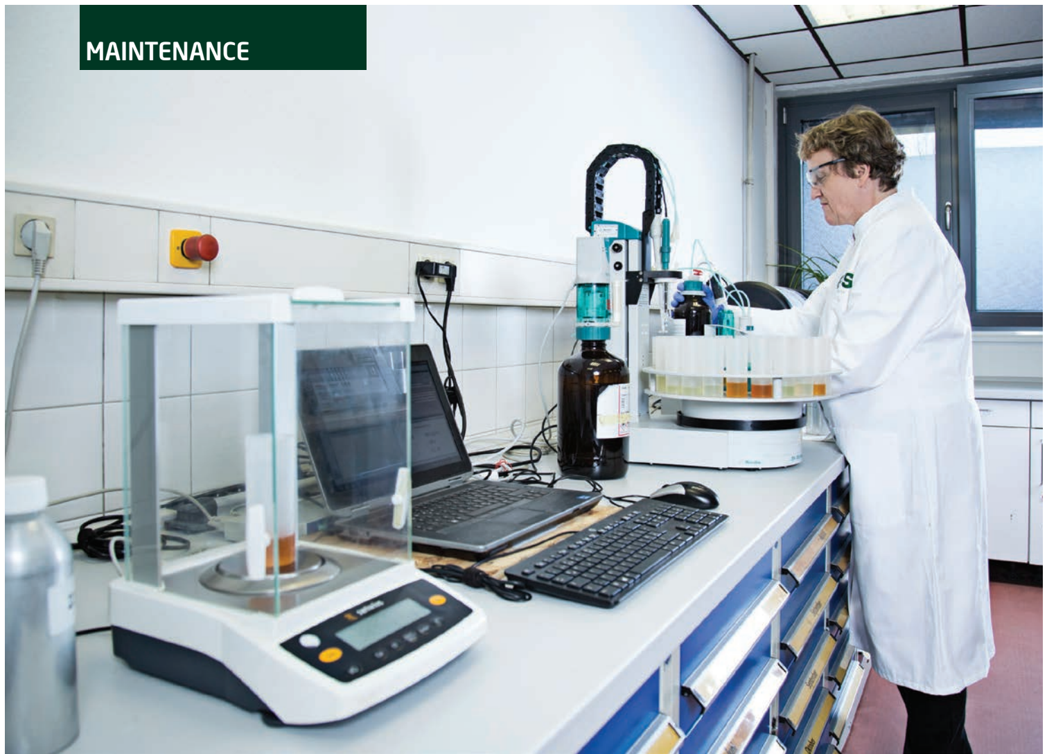
The EOS-owned laboratory allows the testing of different parameters in order to evaluate the insulating oil quality
